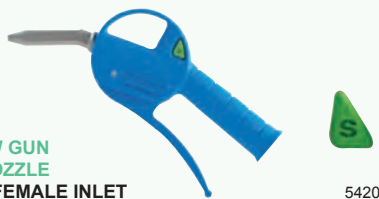
STANDARD LOW PRESSURE BLOW GUN WITH 100 MM STEEL NOZZLE BRASS 1/4" BSP FEMALE INLET
